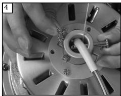
Remove keeper from cross pin and then cross pin from yoke. Replace keeper on cross pin and save.
